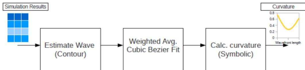
**Figure:** Curvature Estimation of Cardiac Excitation Waves
